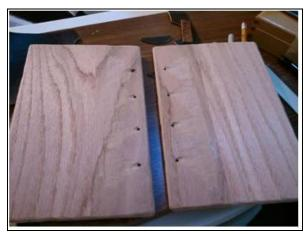
Holes are drilled for the raised cords through the boards at a 45 degree angle to be more ergonomic for the book itself, and increase the overall longevity of the future relic. Divots are sanded so the cords can keep a low profile.
