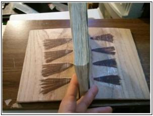
The glue is dry and protective papers are removed. It's as solid as the wood around it.
