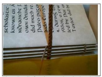
Detail of sewing onto the raised cords. The thread loops around and back through the same hole in the quire.
