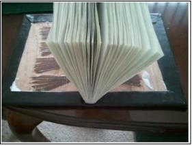
Glue is applied to most of the spine (except for an inch at the top and bottom), the boards are glued, and the book is placed squarely on top of the leather. Edges are folded and trimmed at the corners.
