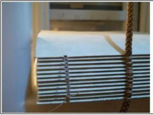
Detail of completed kettle stitches. Also visible is my pencil marking to remind me which way is the top of the book block.
