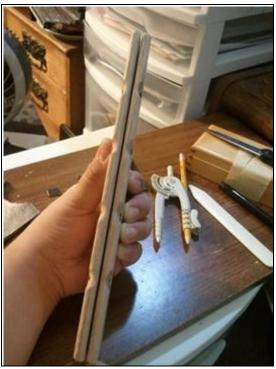
21 The next day I can sculpt, drill, and sand the oak book boards which will become the cover. The boards in the picture above are perpendicular to the camera for showing the thickness, and the divots for the holes that the cords are drawn through so the wood doesn't pinch the cord (pinched cords in a book won't last long).
